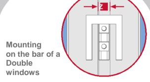
Mount the EM3 sleeve between the window below or above the handle.
